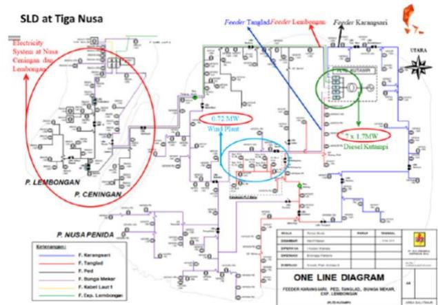
Fig. 4. Single line diagram of the 20 kV distribution grid in Nusa Penida Island [20]
