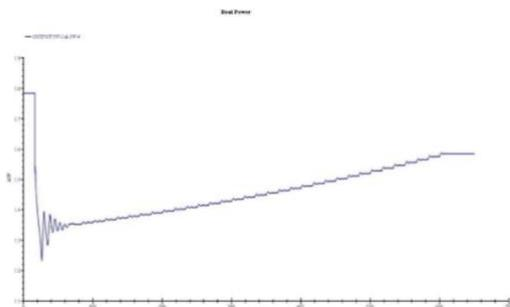
a. Active power output for PV-3 and 4 due to irradiation change – Case 1
