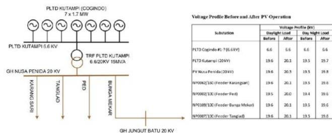
Fig. 7. Single line diagram of Nusa Penida Distribution System (left) and voltage profile before and after PV operation (left). PLTD refers to the diesel power generation plant.
